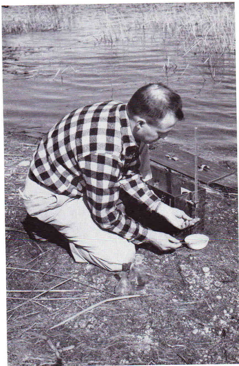
Collection of essential information is facilitated by the use of a field kit equipped for determination of dissolved oxygen, pH, carbon dioxide, alkalinity and acidity.
