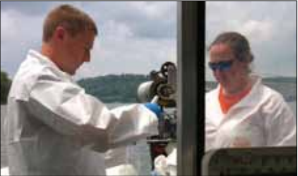
ORSANCO and USGS employees collect water for methyl mercury analysis
