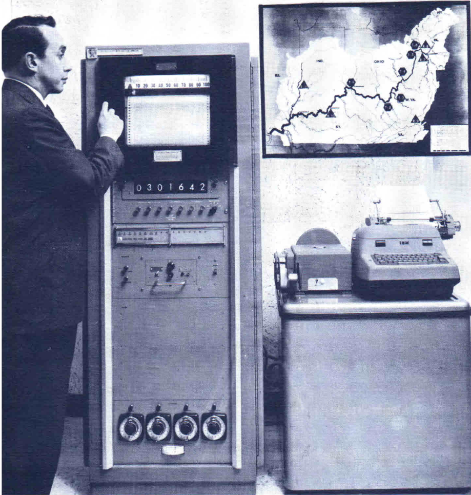
This is the nerve center of the ORSANCO robot-monitor system in Cincinnati. Every hour on the hour the telemeter unit (left) interrogates robot monitors in various locations along the river. Each monitor responds in sequence to report quality conditions. A data-logger (right) transcribes information in tabular form through an automatically operated typewriter, and also makes a punched tape for computer processing of data. Here the equipment is being adjusted by William L. Klein, chemist-biologist of the ORSANCO staff.
