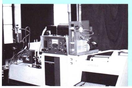
A gas chromatograph is the primary instrument used in the Early Warning – Organics Detection System.
