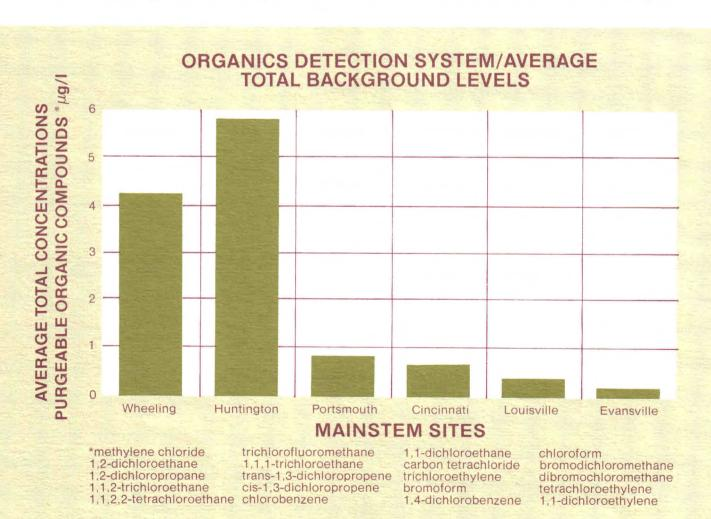
data from the spill detection network are presumptive results only. When unusually high levels of a given material are noted, a sample must be sent to a laboratory for further testing and confirmation. The data from the system must therefore be viewed as tentative; however, certain trends are discernible.
