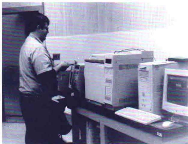
Frank Blaskovich, a Wheeling Water Department operator, uses the new gas chromatograph to check a sample of Ohio River water.
