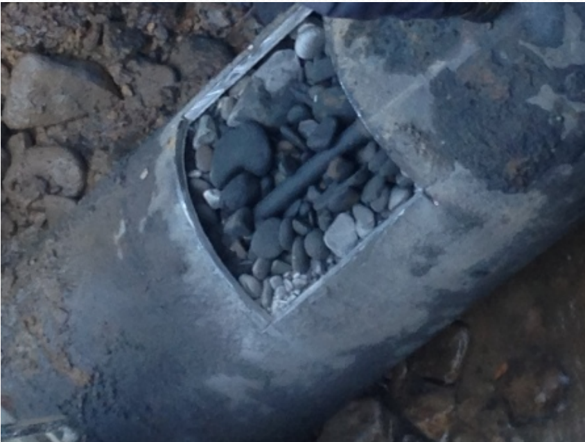
1000 ft of line filed with rock and sand
