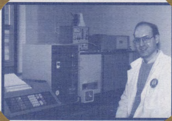
The Organics Detection System provides advanced warning to water treatment facilities when organic substances are detected in the river. This allows for protective measures to be taken to safeguard the water supply.
