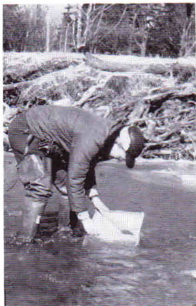
Three types of bottom samplers for streams. A Surber net sampler is shown at top left. The serrated edge of the circular type sampler (top right) is an advantage in cutting into clay bottoms. A Peterson dredge appears in the lower photo, in position to be lowered for a bottom sample.
