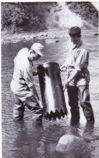
Three types of bottom samplers for streams. A Surber net sampler is shown at top left. The serrated edge of the circular type sampler (top right) is an advantage in cutting into clay bottoms. A Peterson dredge appears in the lower photo, in position to be lowered for a bottom sample.
