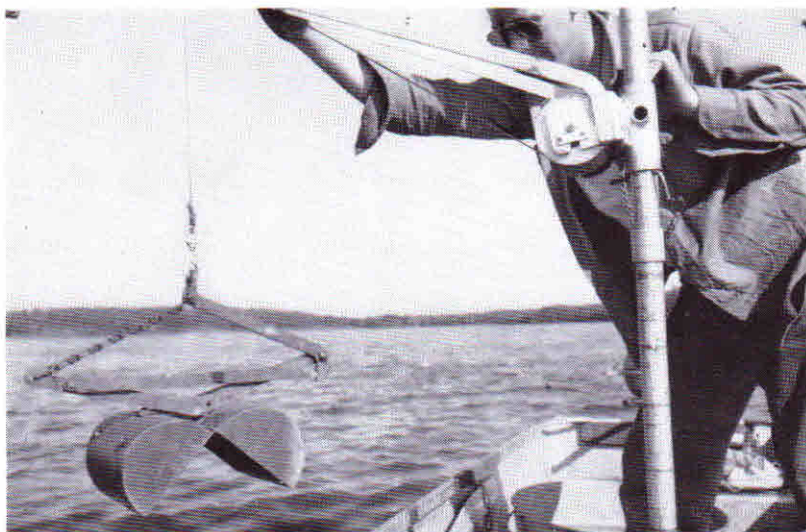
Three types of bottom samplers for streams. A Surber net sampler is shown at top left. The serrated edge of the circular type sampler (top right) is an advantage in cutting into clay bottoms. A Peterson dredge appears in the lower photo, in position to be lowered for a bottom sample.
