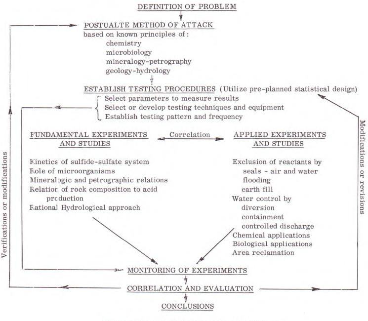
Effects of the overall abatement program of fundamental principles applied to the reduction of acidity in mine waters as measured by specific parameters. Effects at the sources of production Effects in the receiving streams
